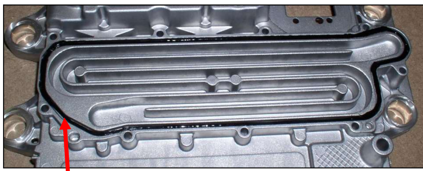
Bottom section with channel filled with sealant
